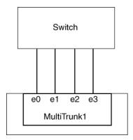
Several technologies exist that enable traffic in a single aggregated link to be distributed across multiple physical switches. The technologies used to enable this capability vary among networking products. Static multimode interface groups in Data ONTAP conform to the IEEE 802.3 standards. If a particular multiple switch link aggregation technology is stated to interoperate or conform to the IEEE 802.3 standards, it should operate with Data ONTAP.
