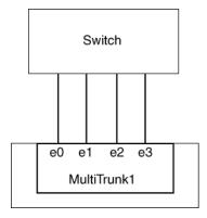
Several technologies exist that enable traffic in a single aggregated link to be distributed across multiple physical switches. The technologies used to enable this capability vary among networking products. Dynamic multimode interface groups in Data ONTAP conform to the IEEE 802.3 standards. If a particular multiple switch link aggregation technology is stated to interoperate or conform to the IEEE 802.3 standards, it should operate with Data ONTAP.
