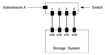
The following figure shows the four network interfaces grouped into a single interface group called Trunk1.
