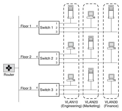
In this figure, VLAN 10 (Engineering), VLAN 20 (Marketing), and VLAN 30 (Finance) span three floors of a building. If a member of VLAN 10 on Floor 1 wants to communicate with a member of VLAN 10 on Floor 3, the communication occurs without going through the router, and packet flooding is limited to port 1 of Switch 2 and Switch 3 even if the destination MAC address to Switch 2 and Switch 3 is not known.
